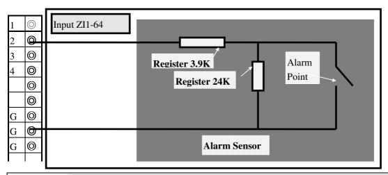
Note: To prevent false alarm and fault also connect 3.9K-ohm resistor To GROUND for unused zones.
